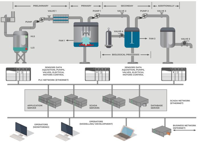
flexibility and capabilities that surpass standard SCADA HMIs. HMI provides high quality graphic visualization, real-time situational awareness and alarm management, enabling operators to efficiently manage/control critical plant operations from central location or remote-control room.
